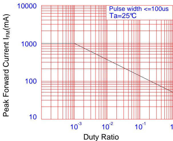
Fig.5 Peak Forward Current vs. Duty Ratio
