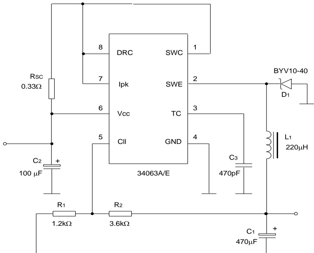
Test Condition ( $V_{OUT} = 5$  V)
