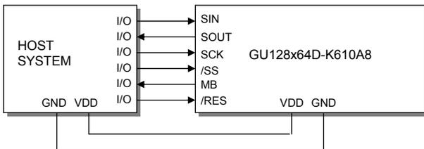
The /SS pin can be used as an enable pin if other devices are connected to the SPI bus. The use of the /SS line is optional, and can be permanently pulled low if not required. This is not recommended since /SS ensures synchronisation of the SPI bus.
