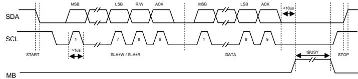
The SCL and SDA lines are internally pulled up with 10K resistors.
