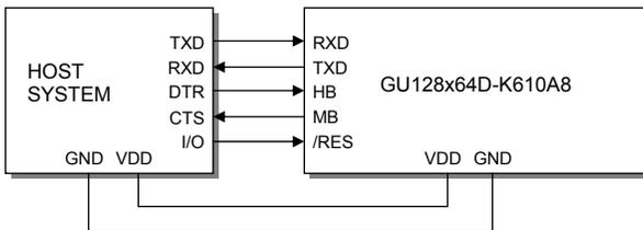
The host busy line (HB) stops the module from sending data to the host until the line falls. The use of the HB and MB lines are optional, and can be connected together if not required.
