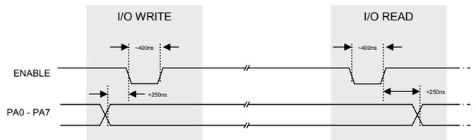
When I/O control is used, the Enable line can be used as an active low read or write strobe. With the I/O read command, the enable line will clock before the module reads the I/O port status. With the I/O write command, the enable line will clock after the I/O lines have been set.
