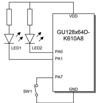
With asynchronous communications enabled, the status of PA0-PA7 can be transmitted when a change in level is detected on any pin. This automatic response mode can be enabled by using the 'UART SETUP' command. When this mode is enabled, the VFD module can reliably check port changes every 15ms. With auto send disabled (default) a manual read command is required to determine the port status.
