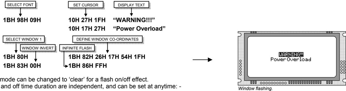
The window mode can be changed to 'clear' for a flash on/off effect. The flash on and off time duration are independent, and can be set at anytime: -
