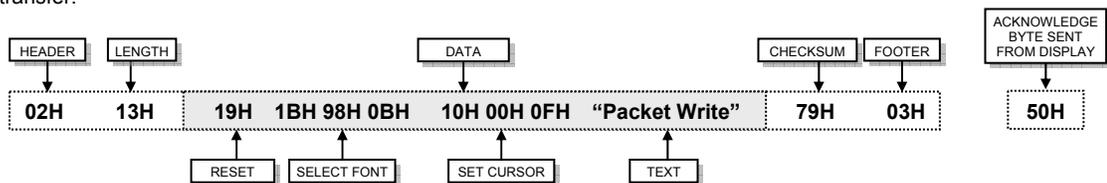
If an error occurs, the display module will discard the data, the host should then re-send the entire packet. If the packet is received correctly, then the data is placed within the 256-byte receive buffer. The receive buffer is enabled automatically when using packet mode.
